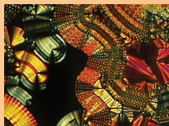
Polarized optical microscopy texture of the prototypical bent-core material with undulated smectic layers. [Antal Jákli, Oleg D. Lavrentovich, and Jonathan V. Selinger, Rev. Mod. Phys. 90 , 045004 (2018)]
