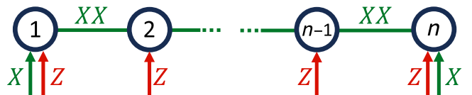
FIG. 1. A linear spin chain of n qubits with nearest-neighbor XX interactions. Single-qubit Z driving and X driving on the end qubits enables efficient preparation of various quantum states, including Greenberger-Horne-Zeilinger (GHZ) and cluster states, and the realization of effective dynamics with multiqubit interactions.
