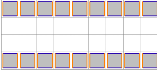
FIG. 6. The patch arrangement considered in this study. Gray patches indicate logical data qubits. The white patches in the middle are used for lattice-surgery routing or ancilla-state injection.
