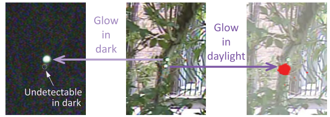
FIG. 1. Imaging demonstration in night and sunlight. A glow-in-the-daylight phosphor disk \text{LuPO}_4:\text{Pr}^{3+} and a commercial glow-in-the-dark phosphor disk \text{SrAl}_2\text{O}_4:\text{Eu}^{2+}, \text{Dy}^{3+} are attached to a tree trunk, as shown in the middle picture. The left picture is taken on a dark night, while the right picture is taken in the daytime. The charged \text{LuPO}_4:\text{Pr}^{3+} nearly does not emit in the dark environment (the location of the phosphor is marked by a dashed circle in the left picture) but exhibits solar-blind ultraviolet emission in the outdoor sunlight environment (the ultraviolet signal is highlighted by a red false color overlay in the right picture).
