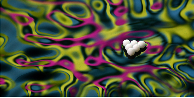
FIG. 1. Oblique perspective of a cluster of six spherical particles, each of radius 0.079 cm, momentarily occupying a triangle configuration in a field of supercritical Faraday waves of characteristic wavelength \lambda = 0.84 cm. The Faraday waves are visualized using a reflected color pattern [14]. The complex fluid environment due to the Faraday waves and horizontal turbulent surface flows plays the role of an active bath.
