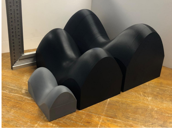
FIG. S1: Image of the three substrates used in the experiments. The grey substrate corresponds to Bo = 102 \pm 1 , while the two black substrates correspond to Bo = 408 \pm 5 and Bo = 725 \pm 9 .
