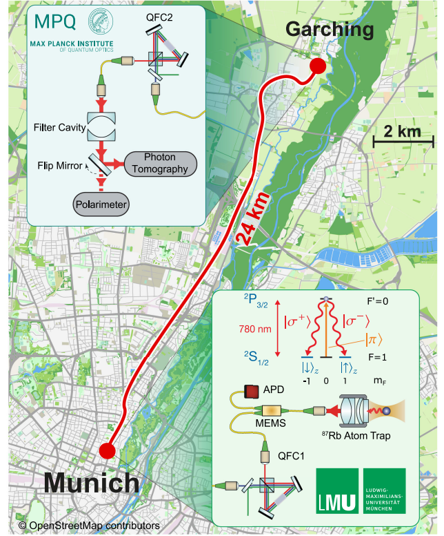
FIG. 1. Metropolitan quantum link. Two laboratories in the greater Munich area are connected via a 24\text{ km} long fiber in order to distribute atom-photon entanglement. The Rb atom at LMU (node 1) is entangled with a photonic qubit (see level scheme), which is subsequently converted to a telecom wavelength at QFC1, propagates 24\text{ km} of fiber, is back-converted to 780\text{ nm} at QFC2, and after spectral filtering is finally measured in a photon projection measurement at MPQ (node 2). After communicating to LMU the arrival of the photon at MPQ, the atomic state is measured via fluorescence readout using a micro-electro-mechanical systems (MEMS) switch and an avalanche photo-detector (APD).
