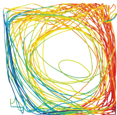
Trajectory of a buoyant sensor's temperature and position in a Rayleigh-Bénard convective flow. Flow temperatures range from 27 °C (violet) to 30 °C (red) at millimeter resolution. See article 234302.
