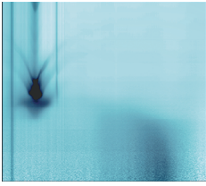
Frequency response of an inductive superconducting single-electron transistor as a function of excitation power (vertical axis); frequency is plotted along the horizontal axis. See article 066805.
