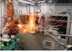
Image of the apparatus used to generate a 110 T magnetic-field pulse exploding, as intended, during operation. Selected for an Editors' Suggestion. [A. Ikeda et al. , Phys. Rev. Lett. 135 , 186702 (2025)]
