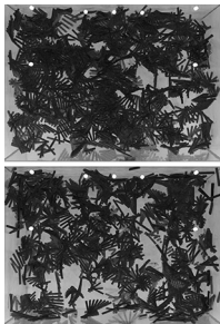
Two stages of cooling of a gas of rod-shaped grains in microgravity. [K. Harth et al. , Phys. Rev. Lett. 120 , 214301 (2018)]
