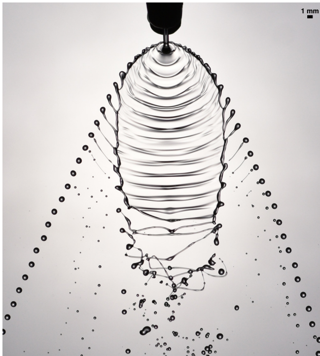
FIG. 1. A stroboscopic front view shows the breakup of a liquid sheet formed by the orthogonal impact of two liquid jets having a diameter of 1 mm. The front jet is visible in the image, while the second jet, being directly aligned behind it, is obscured from view. Atomization occurs through both rim breakup and wave-driven instabilities on the sheet, with visible perturbations originating at the point of impact. The Weber number of the jet is We = 338 , and the Reynolds number is Re = 103 .
