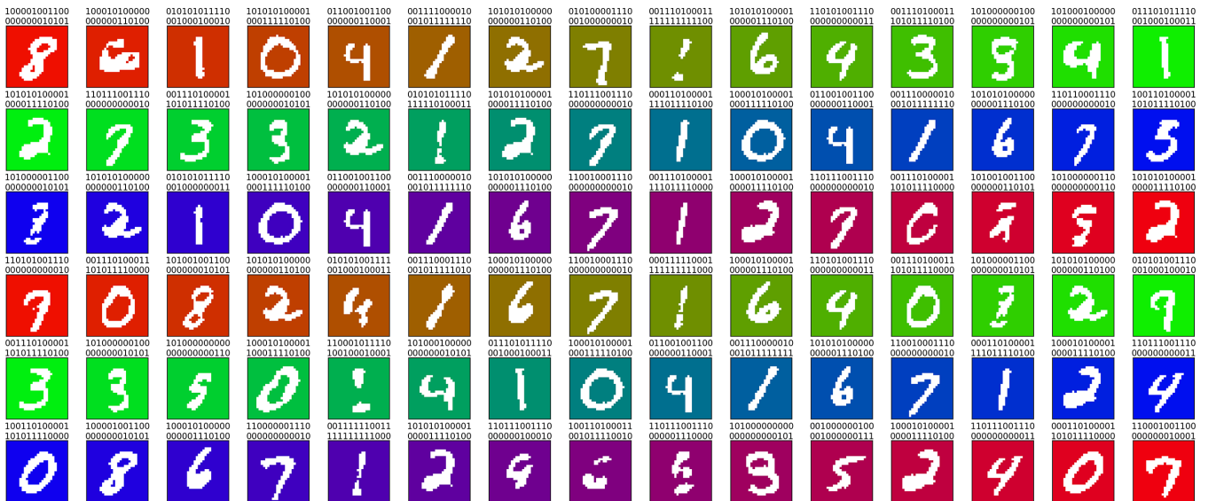
FIG. 6. Markov chain generated by the model shown in Fig. 5. Each panel shows the visible configuration together with the hidden binary pattern that generated it, displayed above the image, which is the digitized average output of that hidden configuration. The sequence progresses row by row and illustrates how digits emerge from combinations of shared hidden features, and confirms that the model is capable of generating sequences of independent digits.
