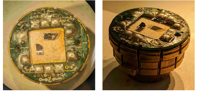
FIG. 9. Two \text{TaNiTe}_5 samples on a standard Quantum Design measurement puck. Note how both of them are held by the gold wires alone, thus floating above the platform.
