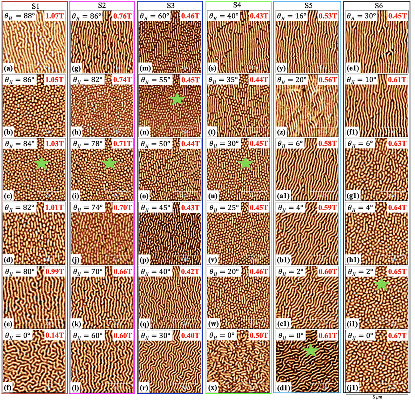
FIG. 2. (a)–(f), (g)–(l), (m)–(r), (s)–(x), (y)–(d1), and (e1)–(j1) represent the angle-dependent MFM images for the Co thicknesses of 8 Å, 10 Å, 12 Å, 16 Å, 20 Å, and 24 Å, respectively, at remanence after applying different DC saturation fields under different angles and reduction to zero according to the protocol described in the main text. All MFM images have the same area-of-view equal to 25 \mu\text{m}^2 .
