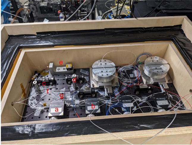
FIG. 5. Photograph of the insulating box hosting the FRR filter, with the upper lid removed. The main constituting components are labeled in red: variable ratio directional couplers at the bus (a) and drop (b) port, polarization controllers (c), (d), piezoelectric stretcher (e), and splices along the fiber-ring path (f), (g). The unlabeled components are not part of the filter setup.
