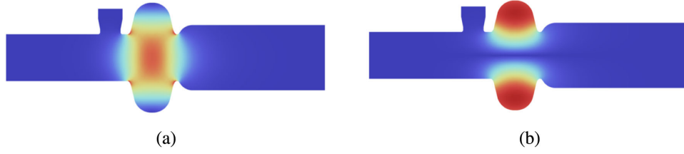
FIG. 18. HALF rf fields. (a) Electric field and (b) magnetic field.
