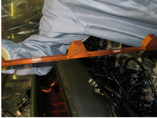
FIG. 21. Discharge between back of the rods and stems of the SARAF RFQ.
