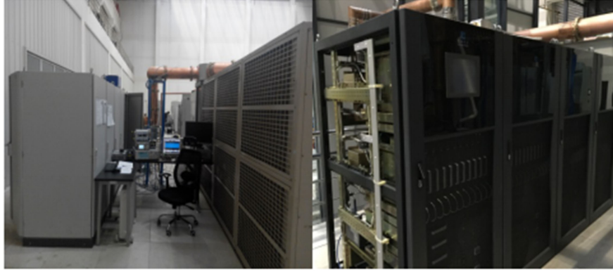
FIG. 26. Tetrode AMP (left) and two 80 kW SSPAs (right).
