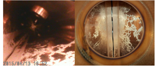
FIG. 19. Vane surface of C-ADS Injector I RFQ nearby coupler and electrode surface opposite to coupler.
