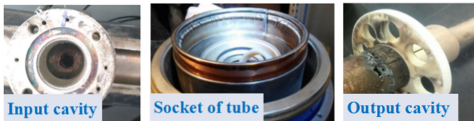
FIG. 25. Input cavity, socket of tube, output cavity of a 200 kW tetrodes amplifier were burned in C-ADS Injector II.
