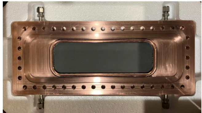
FIG. 14. Photograph of the rf window coated with the DLC on the vacuum side.
