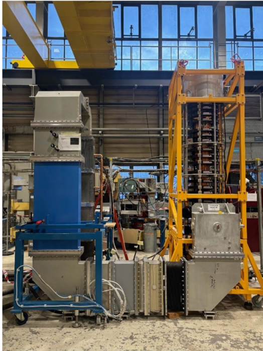
FIG. 18. TH2167HE prototype installed in the CERN test stand.
